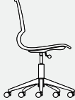
Ⓟ 3530, Ⓡ 3531 Base in alluminio girevole su ruote e pompa a gas / Swivel base in aluminium with castors and gas lift mechanism
